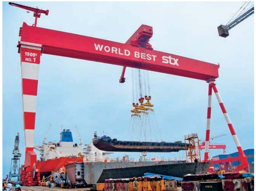
As floating cranes with sufficient capacity and hoisting height are available in Korea, it was actually possible to supply and erect the crane in seven pre-fabricated parts. The rough erection of the crane lasted only 7 days.
