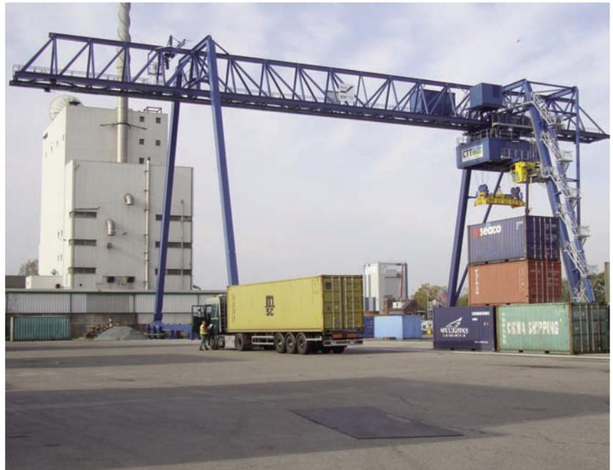
One thing applies to all three Barge Servers: the slewing trolley has double-winch equipment which can be turned around by approx. 305 degrees. It can be moved carefully and precisely to any container position. The driver can always keep an eye on what is going on from the integrated cabin.
