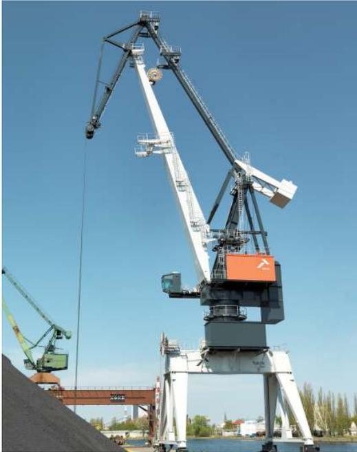
Their new electrically driven TUKAN 1500 is rail-mounted on existing rails and equipped with 4-rope grab hoisting gear. With a cable reel for power feeding and control installed on the jib, assorted lifting attachments such as telescopic spreaders, motorized grabs, magnets, coil clamps and similar can be attached and operated, making this crane a truly versatile multipurpose lifting device.
